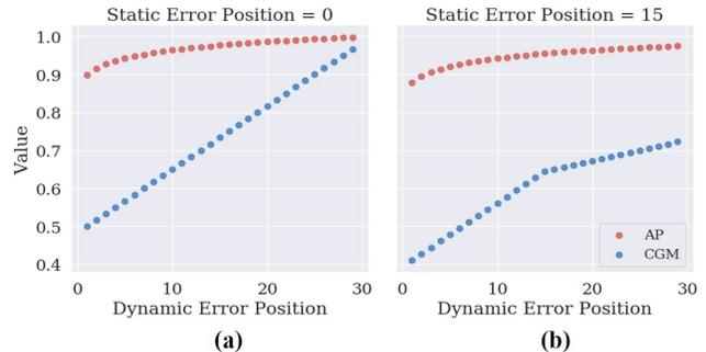
Figure 1. Position-sensitive comparisons between AP and CGM. Assume an original list consisting of 30 correct samples and only one error sample is dynamically inserted into the list. We exhibit: (a) No static error sample (b) One static error sample in the middle position. AP values are not sensitive to the error position and tolerate a few error samples in the list. While CGM values are position-sensitive and also equally transmit the error effects to subsequent samples.
