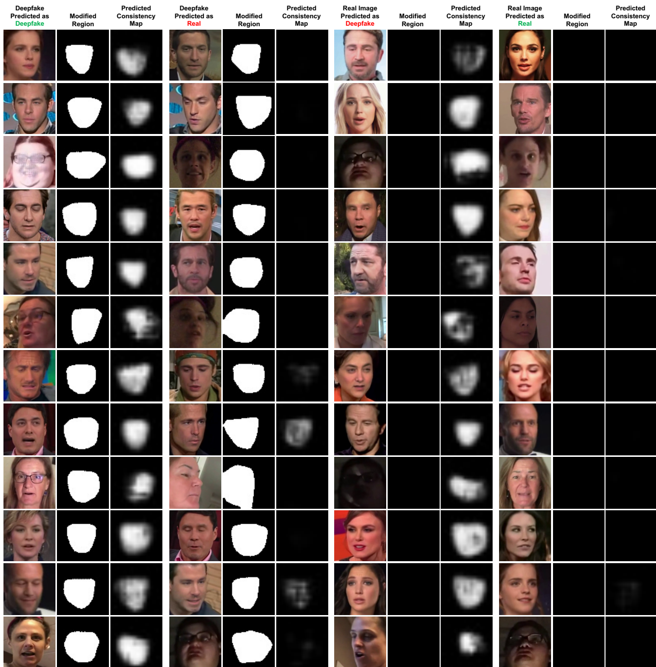
Figure 1: Visualization of the predicted consistency maps \hat{\mathcal{M}} , which try to localize the modified regions. We use the model trained with real videos of FF++ augmented by I2G in the cross-dataset, and the predictions are computed from the predicted consistency volume, as mentioned in Section 3.1 in the main text. The ground truth modified regions are generated by DSSIM, as discussed in Section 4.2 in the main text.
