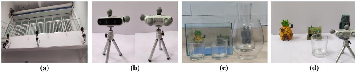
Figure 1. **Tools used in data collecting**(a) Three cameras of motion capture system. (b) the RealSense D435i RGB-D camera with reflective markers. (c) Objects used in the scenes. (d) Typical scene
