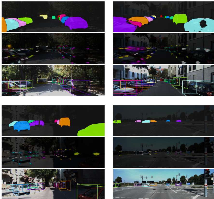
Figure 1: Qualitative results on the KITTI3D test set on Car for the ResNet101 architecture: instance segmentation (top), 2D reference points (mid) and 3D bounding boxes (bottom).
