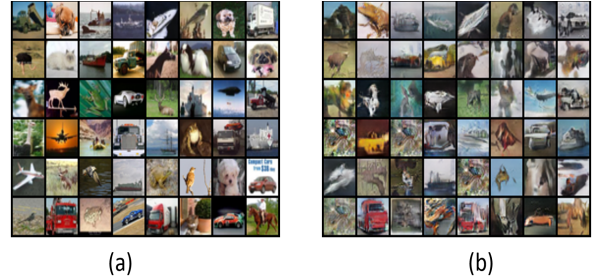
Figure 2. (a) The original images from CIFAR-10 dataset. (b) The corresponding AdvFool images. Though the difference between the AdvFool and original images is visible to human eye, these images still capture the colors and object patterns from the original images.
