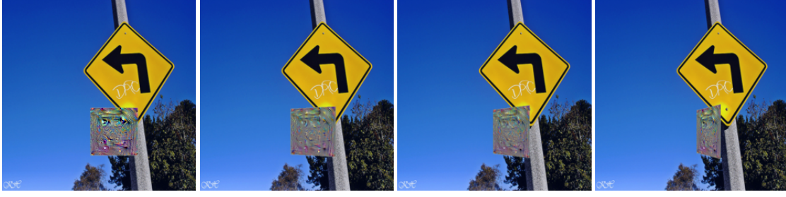
Figure 2. Patches targeting the "mailbox" class inserted into a base image at (left to right) 0°, 20°, 40°, and 60° of yaw.
