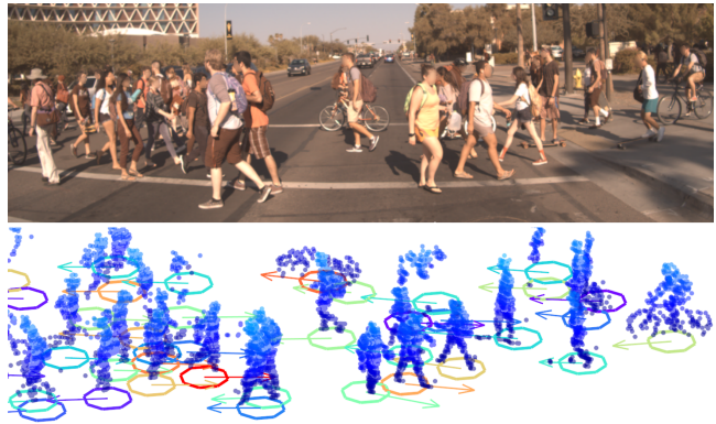
Figure 1. Association and tracking of pedestrians is challenging in dense, urban environments. We propose a real-time learned association and tracking system with IMM filtering that incorporates LiDAR + camera modalities and show improvements on the task of both association and state estimation.
