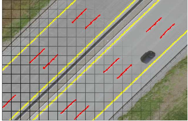
Figure 1. YOLinO detects generic polylines as a bottom-up composition. The image is split into spatial cells each predicting multiple line segments. As one advantage, dashed and solid road markings can be detected using the same head. Aerial image: © City of Karlsruhe | Liegenschaftsamt
