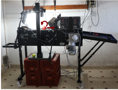
Figure 1. Acquisition system. Upper panel: Machine equipped with a conveyor belt, used for the acquisition of images of apples with a high surface coverage. Lower panel: view of the acquired images of apples after segmentation from the background.
