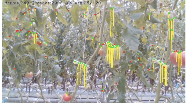
Figure 2. Tracking of the feature points. Green and red dots signify inliers and outliers, respectively. Tracked inlier paths are drawn in yellow.
