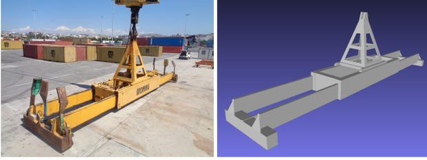
Figure 3. A single-lift crane spreader (left) and its 3D mesh model (right). Note that the three moving gather guides (aka flippers) at each end beam of the spreader have not been modeled.
