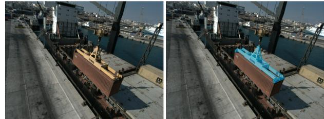
Figure 1. A container hoisted by a spreader (yellow object, left) and a spreader mesh model overlaid semi-transparently in cyan with the pose estimated by the proposed method (right).
