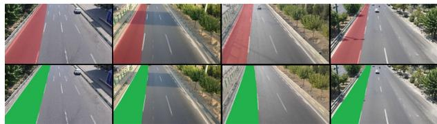
Figure 13. Overtaking lane detection results. The top images represent the predicted overtaking lane by the system in red and the bottom images show the ground truth in green.
