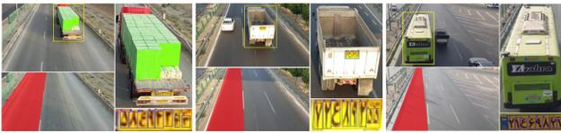
Figure 14. Sample results of the proposed system performance including 4 stages of overtaking lane detection, HGV detection, License plate detection and Character recognition
