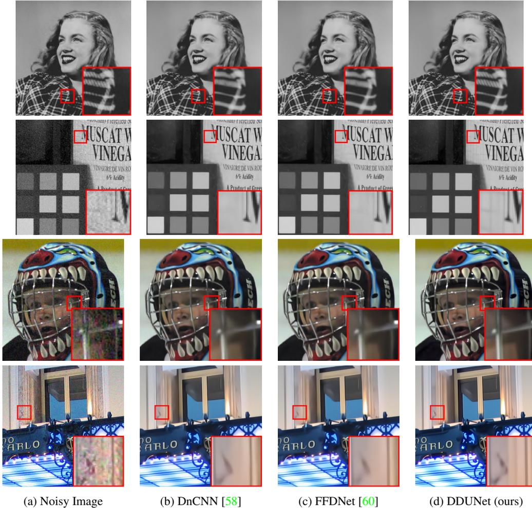
Figure 8: Real noisy image denoising. Left to Right: noisy images, denoised images by DnCNN, denoised images by FFDNet, and denoised images by our DDUNet. We set  $\sigma = 15$  and  $\sigma = 50$  for gray-scale and color images respectively. One can observe that our DDUNet is good at edge recovery and the preservation of the detailed structure.
