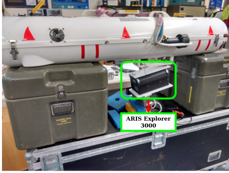
Figure 1: Nessie AUV with mounted FLS sensor (inside the bounding box)
