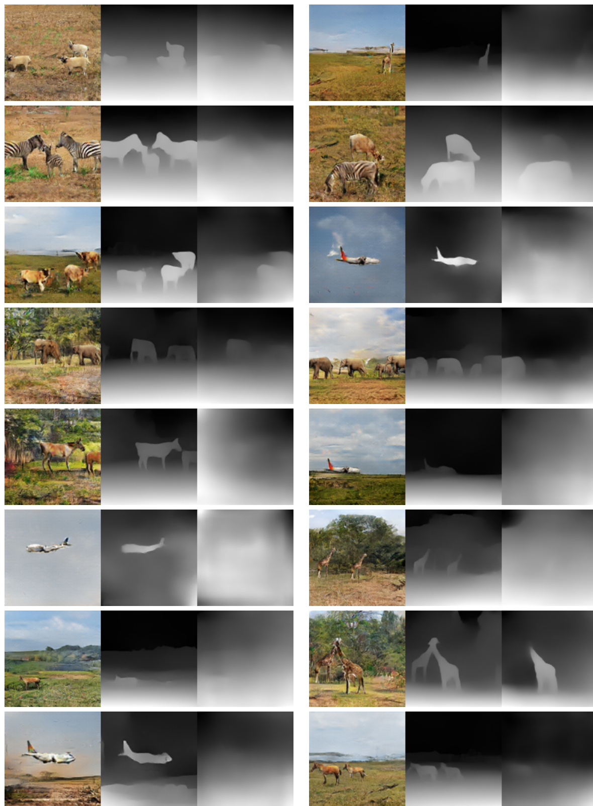
Figure 6. Comparison between the depth maps generated by our method and those obtained by MiDaS. In both columns, from left to right: our generated image, our generated depth map and the depth map computed by MiDaS from our generated image.
