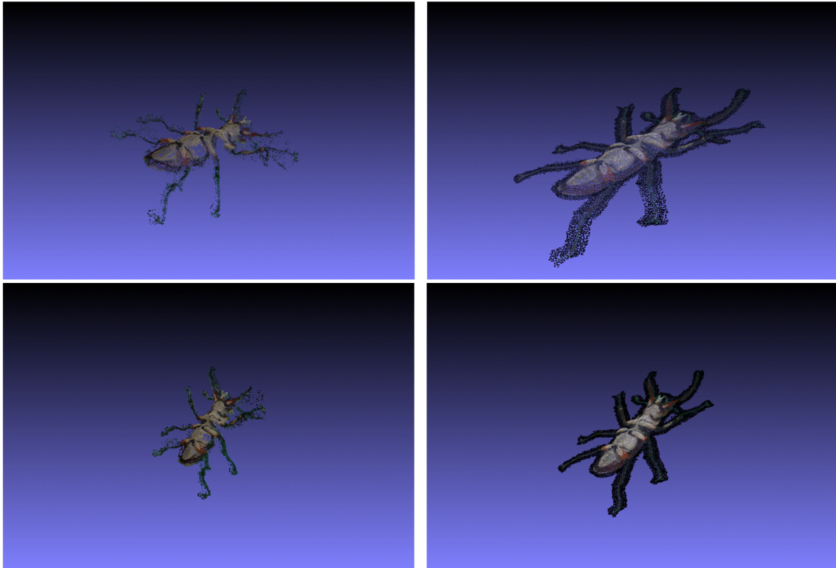
Figure 11. Supplementary SfM reconstructions based on 30 images, see Fig. 1. (Left) SfM reconstruction based on refractive SfM using our method for Scenario 2. (Right) SfM reconstruction based on perspective camera using COLMAP [3].
