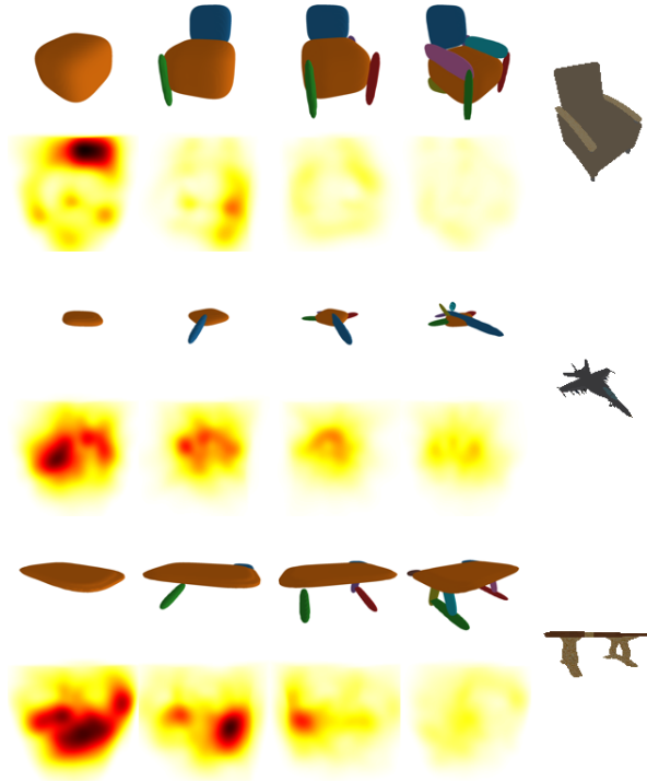
Figure 3: Visualizing ISCO steps. ISCO recomposes the object with a superquadric at a time, going from coarse to fine (top). The gradients of the reconstruction error on the voxel grid inform where to initialize the next one (bottom).
