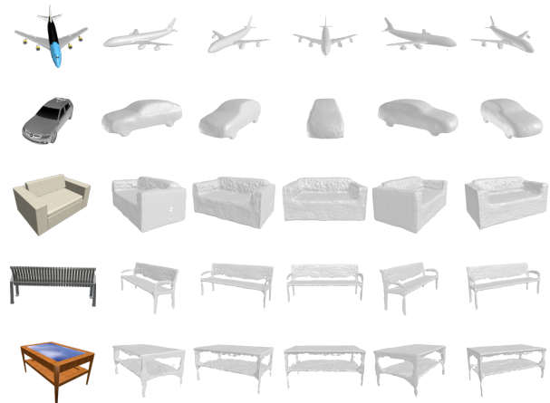
Fig. 1: Five unique views of objects reconstructed by LIST from a single RGB image. Not only does our model accurately recover occluded geometry, but also the reconstructed surfaces are not influenced by the input-view direction.
