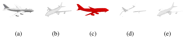
Fig. 3: To evaluate the reconstruction quality of occluded surfaces, we first align the reconstructed shape (b) with the input image (a) and cast rays onto the surface (c). Next, we identify the (red) faces that intersect with the rays via ray-mesh intersection and separate the reconstructed mesh into (d) visible and (e) occluded areas.
