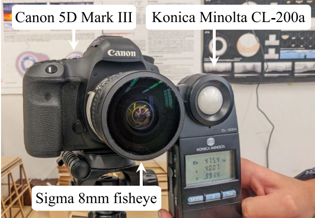
Figure 1. Setup used for the capture of the calibration dataset. The original Canon 5D Mark III camera used for the Laval dataset (left, graciously provided by the original authors) captures a bracket of images at different exposures while the chroma meter CL-200a (right) measures the illuminance and chromaticity of the scene.
