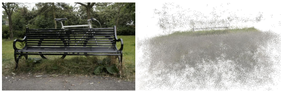
Figure 5: Our method failed on unbounded scenes where noisy points are extracted from the occupancy grid.
