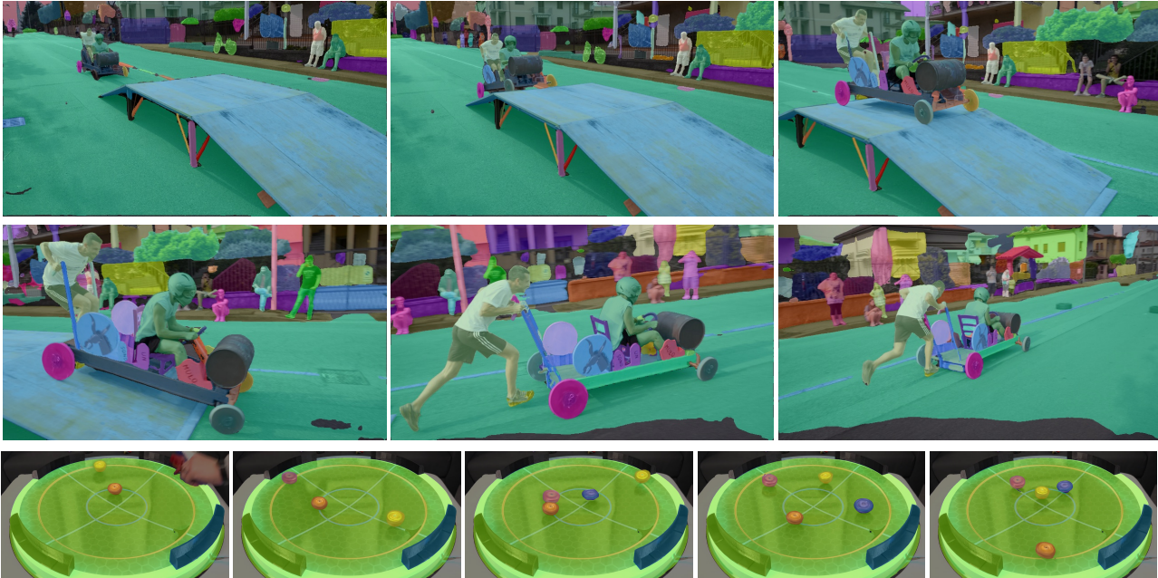
Figure 1. Visualization of our semi-online video segmentation results. Top: our algorithm (DEVA) extends Segment Anything (SAM) [27] to video for open-world video segmentation with no user input required. Bottom: DEVA performs text-prompted video segmentation for novel objects (with prompt “beyblade”, a type of spinning-top toy) by integrating Grounding-DINO [34] and SAM [27].
