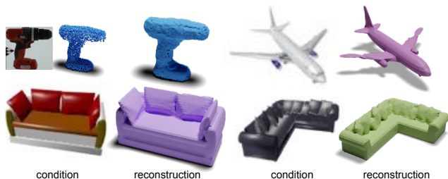
Figure 5. Reconstructing scanned point clouds and single images. Our method captures details of conditioned geometry, such as the curves of the drill, engines of the plane, and pillows on the couch.
