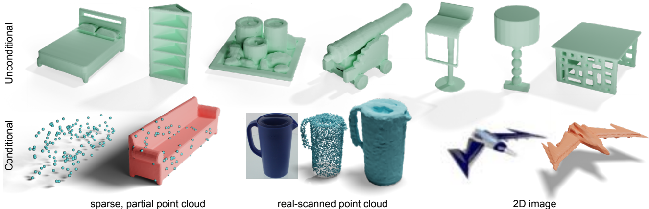
Figure 1. Our method generates clean meshes with diverse geometries. (Top) Unconditional generations from training on multiple classes. (Bottom) Conditional generation given various visual inputs, such as partial point clouds (same point cloud overlaid on sample), real-scanned point clouds, and 2D images. Our method captures details of conditioned geometry, such as the handle of the pitcher.
