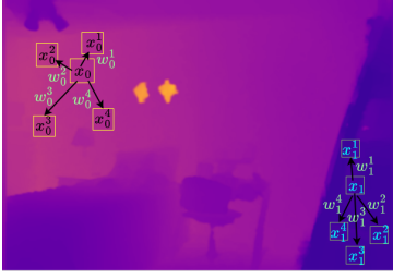
Figure 2. Illustration of the NLAR Module - a non-local extension of classic auto-regressive (AR) model for depth images.
