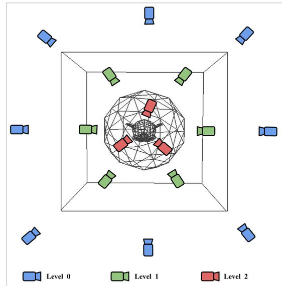
Figure 1. Top, wireframe view of a multi-layered stratified scene with three levels (monkey head inside sphere inside a cube). The camera colors indicate views of a specific level. *Strata-NeRF* enables high-quality reconstruction of such stratified scenes using a single neural network.
