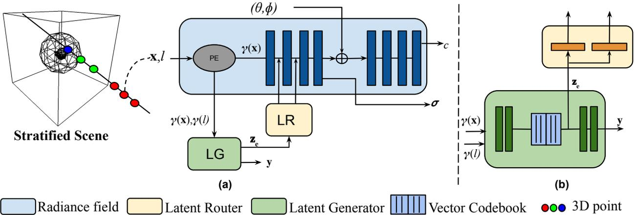
Figure 4. For each 3D point along the projected ray, we generate a latent code using our “Latent generator” module. The generated latent code is routed to the MLP using “Latent Router”. Vector Codebooks learn the discrete distribution of positionally encoded 3D points. (a) Our model’s end-to-end architecture; (b) components of the “Latent Generator” and “Latent Router” blocks.
