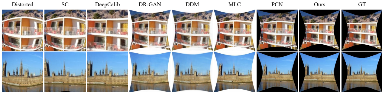
Figure 8: Qualitative results on the synthesized test set. For each comparison, we show the distorted image, the rectified results of SC [48], DeepCalib [6], DR-GAN [38], DDM [39], MLC [37], PCN [58], our method, and ground truth.
