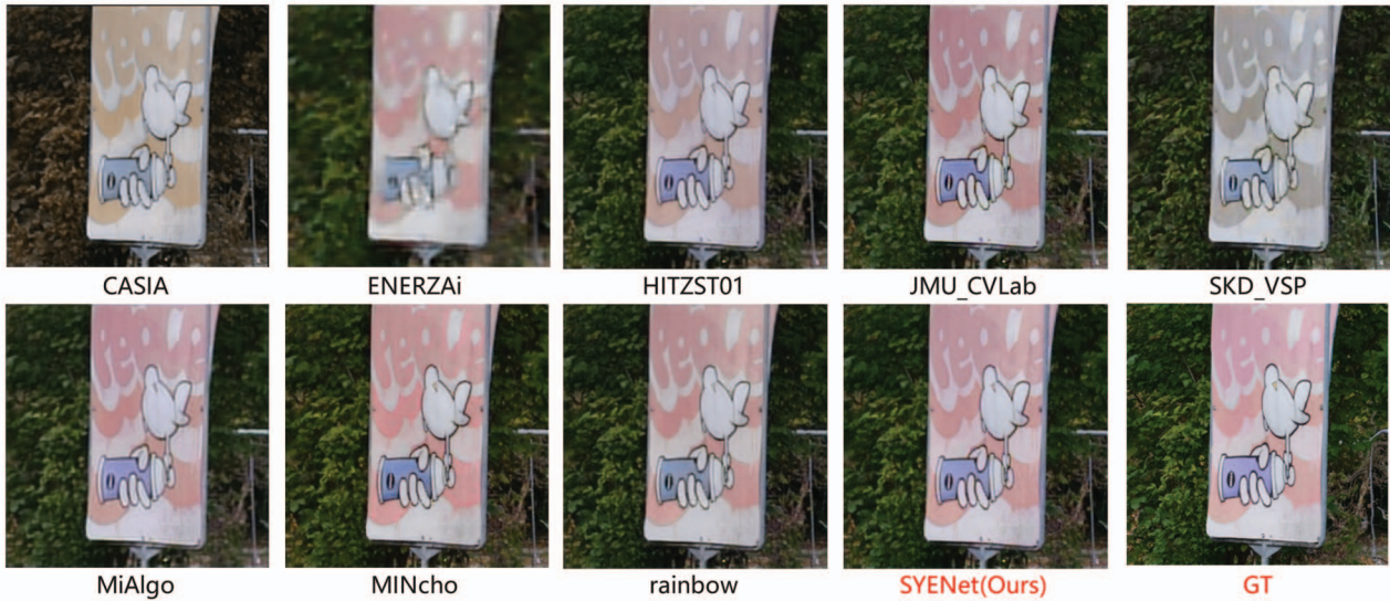
Figure 7: Image signal processing comparisons with models from participants of MAI 2022 Challenge: Our model shows competitive performance compared with other efficient small networks, and the detailed quantitative comparisons are in Table 3. Even though the PSNR of our method is not the highest, the comprehensive performance measured by score (Eq. 9) is the highest. More comparisons of qualitative results are presented in the Appendix J.
