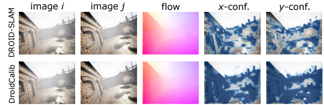
Figure 4. Exemplary estimated flow \mathbf{f}_{ij} and confidence weights \mathbf{w}_{ij} in x - and y -direction (blue overlay) in the last update iteration k . Compared to DROID-SLAM (top), DroidCalib (bottom) predicts higher, less spatially confined confidence weights.
