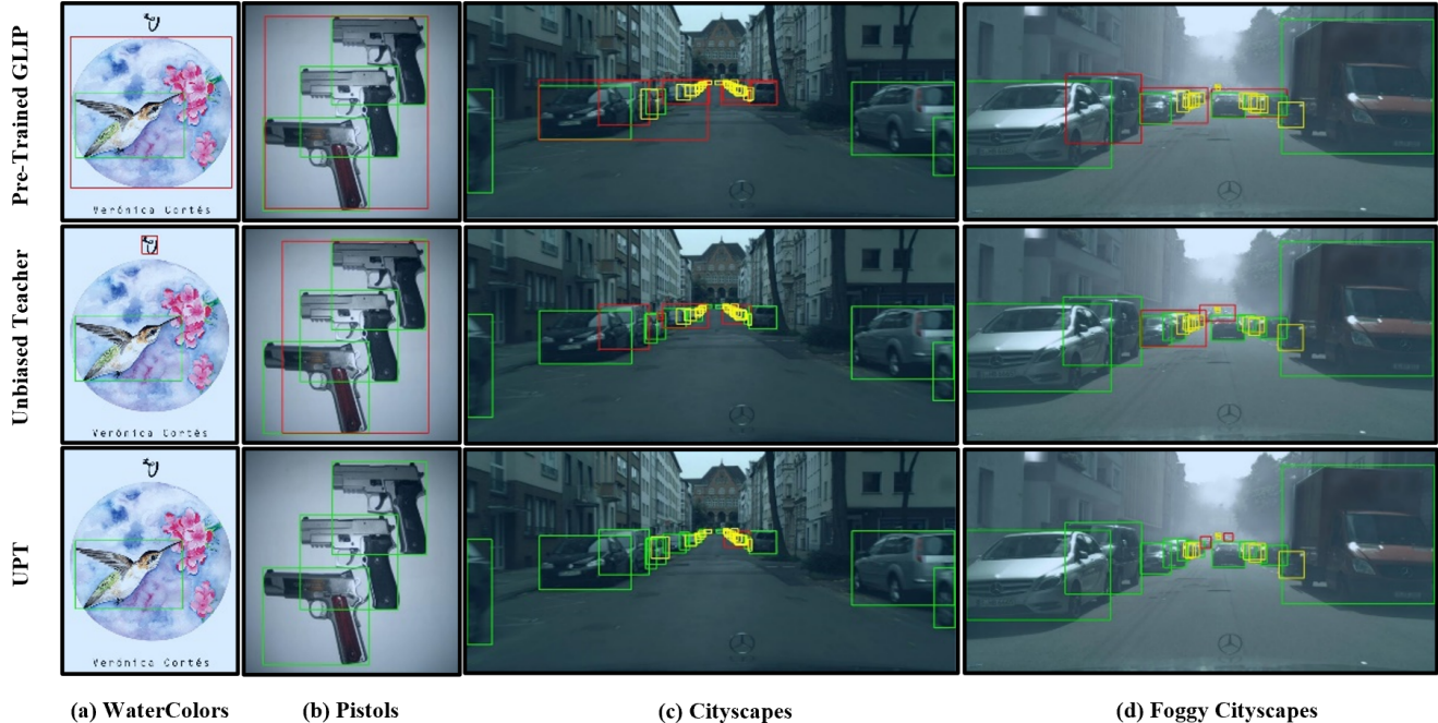
Figure 7: Qualitative results on the downstream tasks. From left to right : WaterColor, Pistols, Cityscapes, Foggy Cityscapes. From top to bottom : zero-shot inference of GLIP-T, Unbiased Teacher, UPT (Nested Mean Teaching + Dual Complementary Teaching). Green , red and gold boxes denote true-positives , false-positives and false-negatives , respectively.
