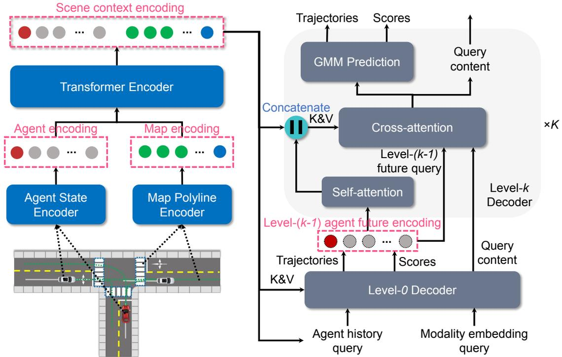
Figure 2. Overview of our proposed *GameFormer* framework. The scene context encoding is obtained via a Transformer-based encoder; the level-0 decoder takes the modality embedding and agent history encodings as query and outputs level-0 future trajectories and scores; the level- $k$  decoder uses a self-attention module to model the level- $(k - 1)$  future interaction and append it to the scene context encoding.
