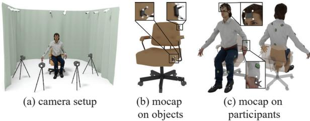
Figure 3: **Setup for data collection in the CHAIRS dataset.** Our data collection setup consisted of (a) four front-facing RGB-D cameras supplemented by a network of motion capture cameras surrounding the recording area, (b) hybrid trackers affixed to various movable parts of objects, and (c) a configuration incorporating five hybrid trackers and seventeen IMUs distributed on the participants.
