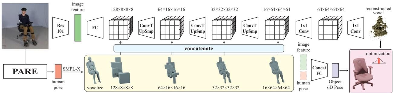
Figure 5: **Model architecture.** The reconstruction model leverages the predicted voxelized representation of the human to facilitate the estimation of pose for the interacting object. We undertake root 6D pose regression for the object utilizing the image feature in conjunction with SMPL-X parameters. The predictions along with an interaction prior are harnessed for the refinement of the final estimated pose.
