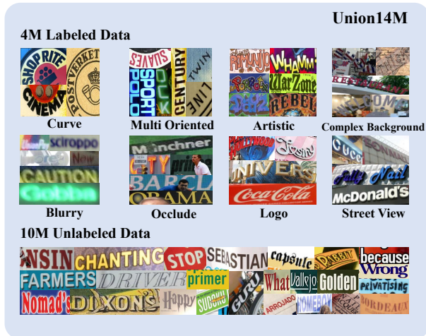
Figure 3. An Overview of Union14M which is used to analyze STR models in real-world scenarios. Union14M contains 4M labeled images (Union14M-L) and 10M unlabeled images (Union14M-U), which cover a wide range of real-world scenarios with intense diversity and complexity.
