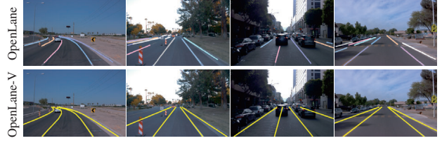
Figure 8. In OpenLane [27], only visible lane parts are annotated, so the same lane may be split into multiple parts. In contrast, in OpenLane-V, each lane is seamlessly annotated, and invisible parts are inpainted. It is recommended to watch the accompanying video to see the improved annotations.
