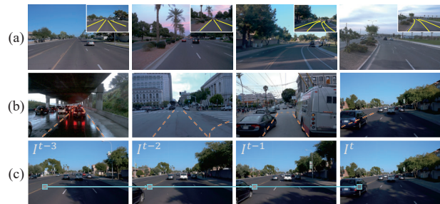
Figure 1. (a) For lane detection, it is required to identify visible lane pixels, represented by yellow lines in the insets. (b) Due to occlusions by nearby vehicles or glistening conditions on wet roads, lanes may be unobvious, which are depicted by orange dotted lines. Besides, lanes may not be marked at crossroads. (c) In a current frame I^t , which is also the rightmost one in (b), some lane parts are occluded by a vehicle but visible in past frames. By utilizing visual cues along the temporal axis, depicted by cyan arrows, we can localize the implied lane parts more reliably.
