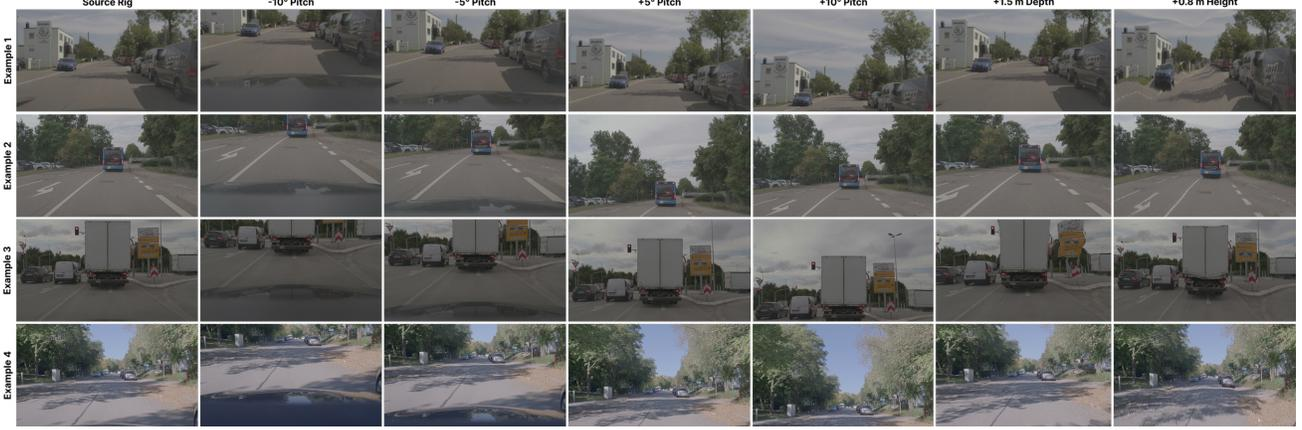
Figure 6. **Novel View Synthesis Qualitative Results:** Shown above are the novel view synthesis results (rectified) obtained with our method. We transform images from the source rig to each of the target viewpoints and then use them for BEV segmentation training.
