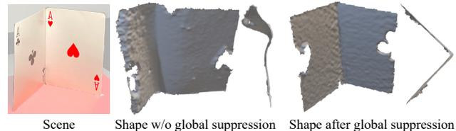
Figure 1: **Structured light 3D scanning using a position sensing diode.** Computational position sensors can enable high-speed, high-resolution 3D imaging at low power and compute budgets. However, global illumination effects such as interreflections in a V-groove significantly bias the measurements, as seen in the poor surface reconstruction in the middle. We propose methods that are robust to such effects, enabling the high-fidelity reconstruction on the right.
