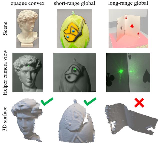
Figure 5: **Global illumination significantly affects the surface reconstructions.** The second row shows the scene from a helper camera view to illustrate such global effects. In the first two columns, the bust and candle are faithfully reconstructed, despite the candle’s subsurface scattering as that effect does not bias the measurements. However, long-range interreflections between the playing cards significantly bias the measurements, causing an erroneous reconstruction.
