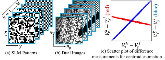
Figure 7: **Robust centroid estimation.** Our method displays masks on the SLM (a), captures the corresponding PSD measurements ( $V_s$  dual image shown in (b)), and performs a linear regression technique to estimate the centroid of the directly illuminated spot. In (c), we plot the pairwise differences of real data using Eq. (15) to illustrate the linear relationship (see text for details).
