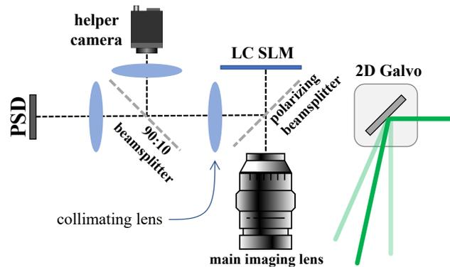
Figure 6: **Optical schematic.** The main imaging lens focuses the scene onto the SLM. The PSD images the masked scene on the SLM. A helper camera views the scene for calibration and ground truth depth experiments.
