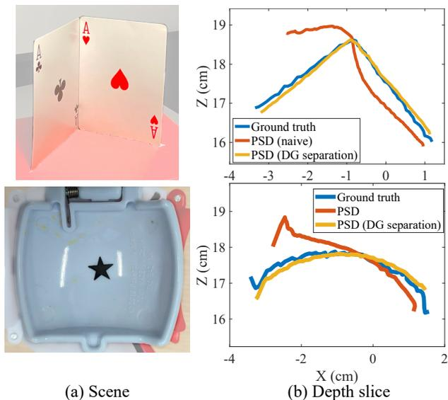
Figure 11: **Effectiveness of global illumination suppression.** A line scan of two scenes with strong interreflections demonstrates our method’s robustness to global illumination. Each object’s concave shape creates large, systemic centroid errors, resulting in erroneous depth estimates (red). In both scenes, our proposed method (yellow) closely tracks the ground-truth depth obtained using the helper camera.
