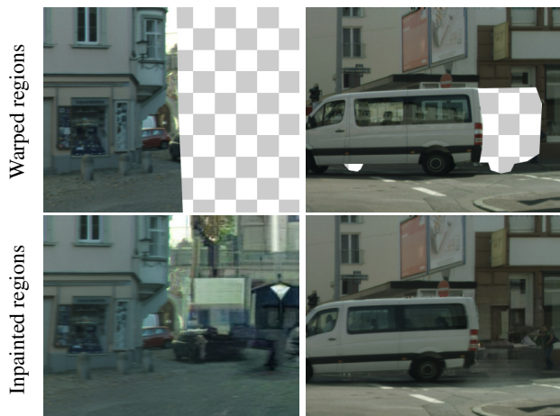
Figure 11. Visualization of the synthesis process: warped visible regions and inpainted disoccluded ones between T and T+10 .
