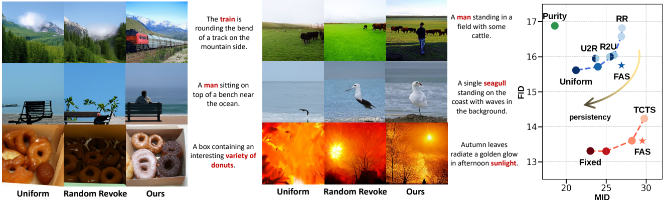
Figure 1: Generated samples on MS-COCO dataset and evaluation graph of various sampling methods showing their trade-off. Uniform sampling is a fixed strategy with notably poor text alignment compared to other methods (FID-40K: 15.61, MID-L: 21.23). Random revoke sampling is a revocable strategy with improved text alignment (FID-40K: 16.81, MID-L: 26.98). Ours is TCTS combined with FAS, where both the image quality and the text alignment are significantly better compared to those of baselines (FID-40K: 13.6, MID-L: 29.5). Metrics are measured on all 40K images with their corresponding single caption. The classifier-free guidance scale was fixed at 5 for all sampling methods.
