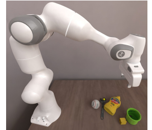
Figure 4: Illustration of the PickClutter task. Given the name of a target object, the robot agent needs to decide whether the corresponding object is graspable based on the current visual observation.
