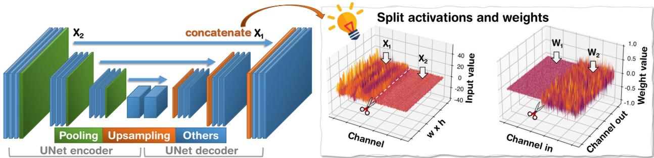
Figure 7: (Left) The typical UNet architecture with shortcut layers that concatenate features from the deep and shallow layers. (Right) The ranges of activations from the deep ( $X_1$ ) and shallow ( $X_2$ ) feature channels vary significantly, which also results in a bimodal weight distribution in the corresponding channels.
