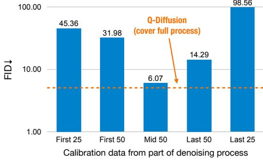
Figure 4: Effects of time steps in calibration dataset creation on 4-bit weights quantization results with DDIM on CIFAR-10. First  $n$ , Mid  $n$ , Last  $n$  denotes that 5120 samples are selected uniformly from the first, middle, last  $n$  time steps.
