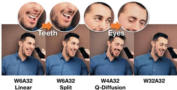
Figure 12: Examples of text-to-image generation with a quantized Stable Diffusion model. Naive linear quantization degrades the appearance of teeth, which gets fixed by shortcut splitting. Q-Diffusion further improves the semantic consistency of eyes through calibration.
