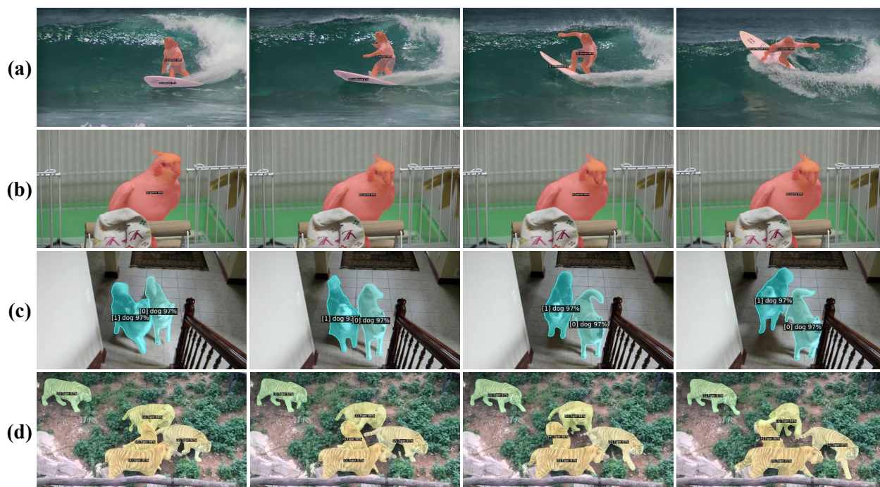
Figure 4. Qualitative results of TCOVIS in four challenging cases on YouTube-VIS 2019 [37] and OVIS [24]: (a) fast movement, (b) heavy occlusion, (c) low resolution, and (d) crowded scene. Objects displayed in the same color denote the same instance. The qualitative results demonstrate the effectiveness and robustness of TCOVIS (Best viewed in color).
