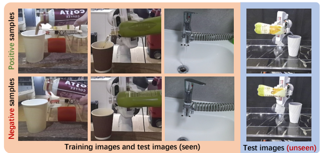
Figure 2. The exemplar of our proposed PourIt! dataset. It includes images with liquid and non-liquid, totaling 3354 training images, 374 seen test images, and 336 unseen ones.
