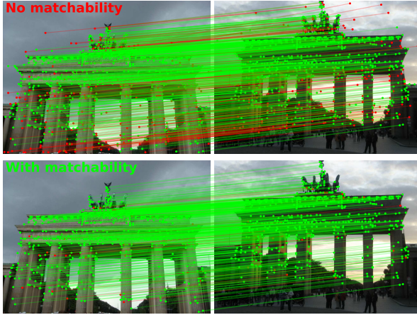
Figure 6. Benefit of the matchability. The matchability helps filter out outliers (red) that are visually similar, retaining only inlier correspondences (green).
