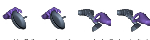
Figure 10: Failure modes of our method. Each pair displays a sample from dual views. The left side shows a generated grasp appears to be more of a touch rather than a proper grasp. The right side shows an unsatisfactory grasp when the sampled ContactGen is infeasible on out-of-domain objects.
