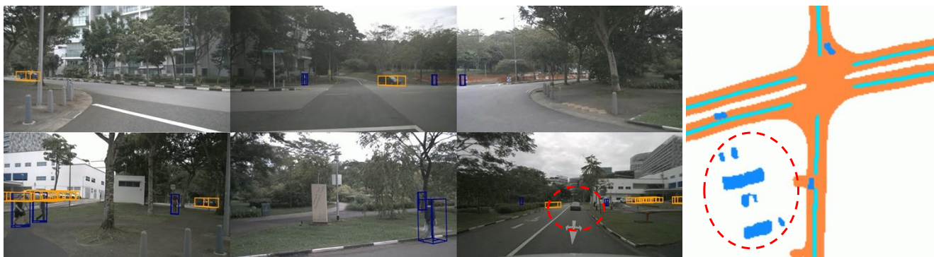
Figure 7. Qualitative analysis of 3D object detection and BEV segmentation. The score threshold of detection is 0.25. The red circles are some failure cases, such as distant objects and blurred borders.
