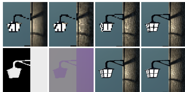
Figure 2. Example of data modalities available in the QRISP dataset. First row, from left to right: Native 270p, Negative 2 mipmap biased 270p, Negative 1.58 mipmap biased 360p, Negative 1 mipmap biased 540p. Second row, from left to right: 540p depth, 540p motion vectors, Native 1080p, Enhanced 1080p
