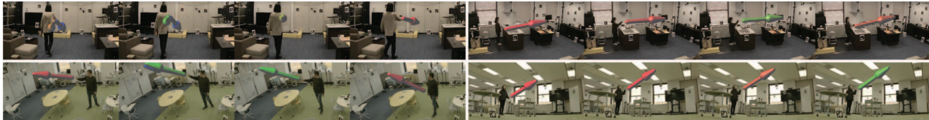
Figure 1. We introduce DeePoint, a neural pointing recognition and 3D direction estimator. DeePoint trained on our newly constructed DP Dataset recognizes when a person is pointing and estimates its 3D direction from video frames captured from a fixed-view camera. Each arrow depicts the pointing direction and its color is green when the person is pointing, red when not. DeePoint successfully recognizes when a pointing starts and ends and can estimate its 3D direction from the complex spatio-temporal coordination of the person’s body.
