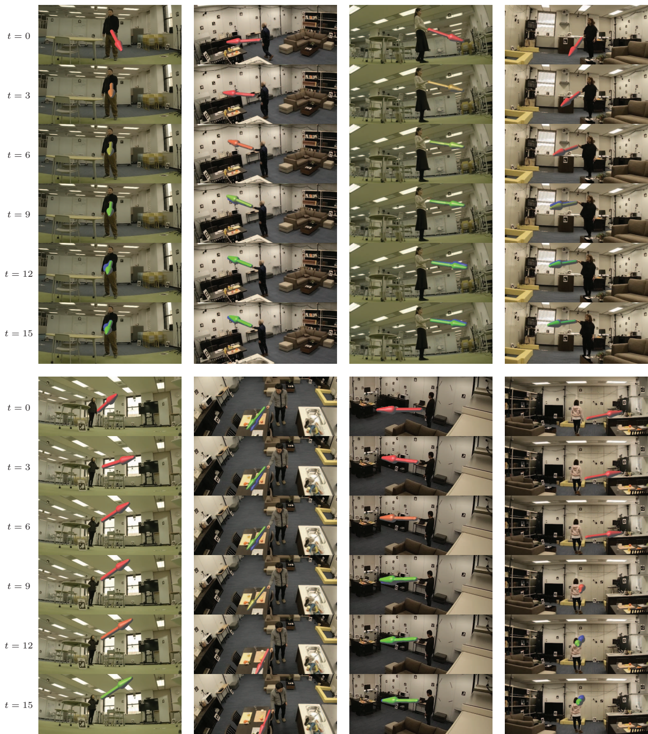
Figure 8. Pointing direction estimation by DeePoint trained with Split-T (i.e., DP ). In each image, the blue arrow denotes the ground truth direction and the other arrow denotes the estimated 3D direction by DeePoint. The color of the prediction arrow represents the result of pointing action recognition. It is green when the person is pointing ( p = 1 ), red when not ( p = 0 ), and gradually transitions between the two colors based on estimated probability. Note how DeePoint correctly recognizes the timing of pointing. For instance, it learns to recognize when the person looks away as the finish of pointing and finds the onset of pointing from change in speed of the movements of the body coordination.
