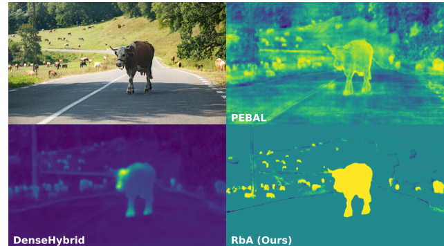
Figure 1: Preserving objectness and eliminating noise. While state-of-the-art methods PEBAL [65] and DenseHybrid [25] suffer from a lack of smoothness and objectness with high false positive rates, our method RbA clearly segments the unknown objects and reduces false positives by eliminating uncertainty at semantic boundaries and in ambiguous background regions.
