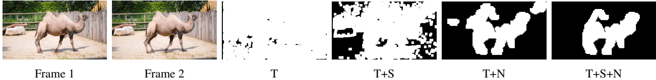
Figure 6: We increase update sparsity using noise suppression and region of interest scaling. T uses the original truncation implementation of DeltaCNN. Scaling the Delta further away from the region of interest ( T + S ) slightly increases sparsity. Using noise suppression ( T + N ) to eliminate single pixel updates increases sparsity even further. Combining scaling and noise suppression ( T + S + N ) achieves the highest sparsity, capturing only the most important updates of the moving camel. Note that in all cases, we dilate the update mask by 10 pixels; explaining the low sparsity in case T . Source: DAVIS 2017
