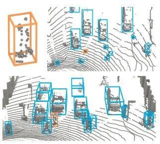
Figure 1. Context matters: a baseline detector struggles at detecting true positive objects confidently if the sampling pattern is atypical, *e.g.* the occluded pedestrian in the orange bounding box (close-up top-left). GACE exploits the geometric properties of the detection and its surrounding objects to significantly increase the score for this detection, which is intuitively correct for a human observer considering this scene.
