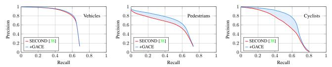
Figure 4. Precision-recall plots for a SECOND [38] model as base detector with and without our confidence enhancement module on the Waymo Open Dataset [33] validation set for LEVEL\_2 APH. Especially at higher recall levels, GACE's better separation of true and false positives leads to higher precision.
