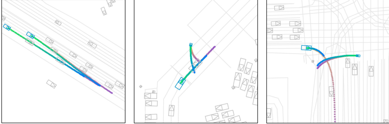
Figure 3. Displayed are the top two predicted joint rollout modes for three WOMD scenes. Color gradients indicate time progression from t = 0s to t = 8s , with the greatest probability joint mode transitioning from green to blue and the secondary joint mode transitioning from orange to purple. Three types of interactions are observed: an agent in the adjacent lane yields to the lane-changing agent according to the timing of the lane change (left), a pedestrian walks behind the passing vehicle according to the progress of the vehicle (center), the turning vehicle either yields to the crossing cyclist (most probable mode) or turns before the cyclist approaches (secondary mode) (right).
