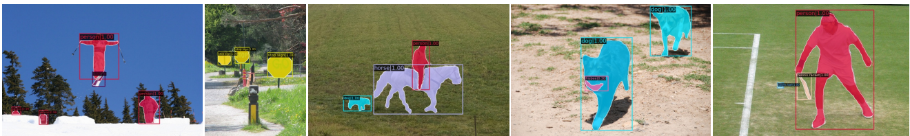
Figure 4: Results on COCO. Examples for object detection and instance segmentation on the COCO 2017 validation set. Our SwiftFormer-L1 model can accurately detect and segment instances in images.
